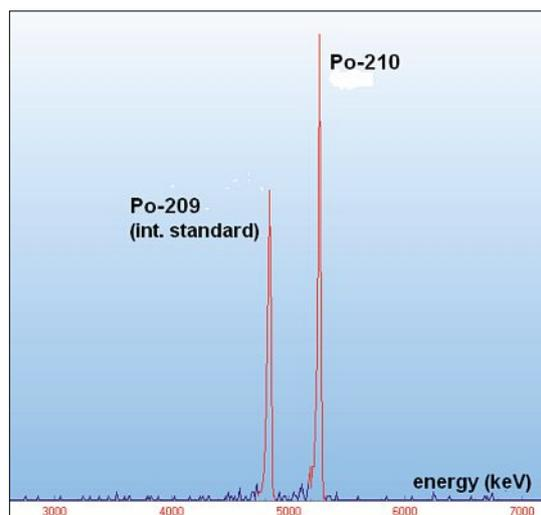
Alpha spectrum of a healing earth extract. For quantification control <sup>209</sup>Po was added (70 mBq). <sup>209</sup>Po has an alpha energy of 4'800 keV. The sample was counted for 24 h in an alpha vacuum chamber (silicon barrier detector).
