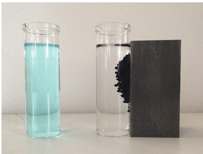
Fig. 7. Adsorption of \text{Cu}^{2+} ions on magnetic chitosan particles (left panel) and adsorption kinetics of \text{Pb}^{2+} on a commercial resin and on Laminaria digitata (marine algae) particles (right panel).
