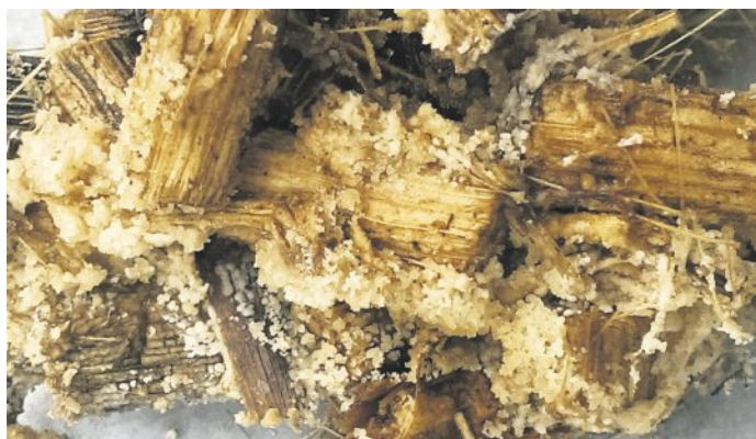
Fig. 4. Used filter material composed of corn stalks and crystallized ammonium phosphate.
