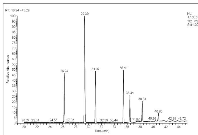
Standard solution containing 2 ppm of each fatty acid methyl ester (compare with the data given in the Table). The signal at 29.39 minutes is the internal standard (d33 - methyl-margarate)
