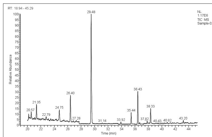
Real Jet A-1 sample showing a total amount of 5 ppm FAME. The signal at 29.48 minutes is the internal standard (d33 - methyl-margarate)
