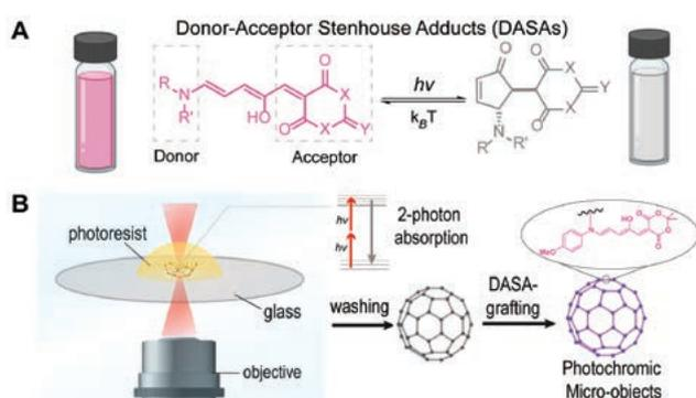
Fig. 1. **(A)** General structures for DASAs and their photoswitching between the open triene (colored) and the closed cyclopentenone (colorless) isomers. R/R': alkyl or aryl; X: O or N. **(B)** Two-photon 3D micro-printing of DASA-containing photochromic micro-objects.
