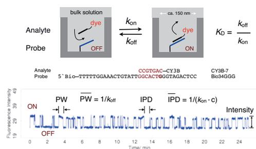
Fig. 1. Experimental setup and a resulting pulse sequence.
