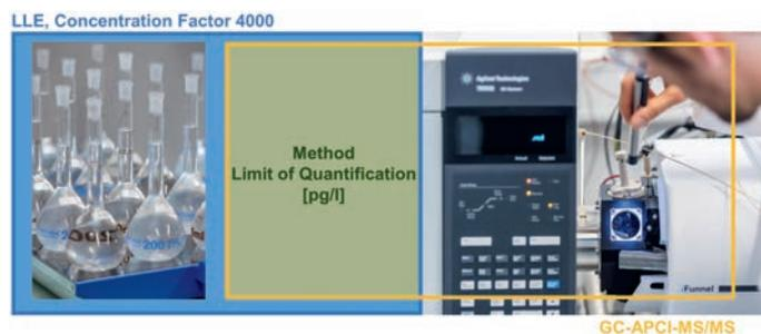
The combination of gas chromatography (GC) with chemical ionization under atmospheric pressure (APCI) and tandem mass spectrometry (MS/MS) allows for ultrasensitive quantification (pg/l) of insecticides. Photos: Alessandro della Bella, Eawag.
