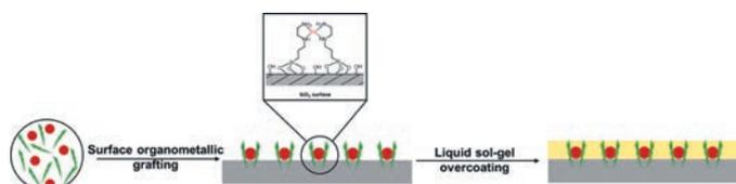
Fig. 1. Synthesis pathway of overcoated palladium catalysts.
