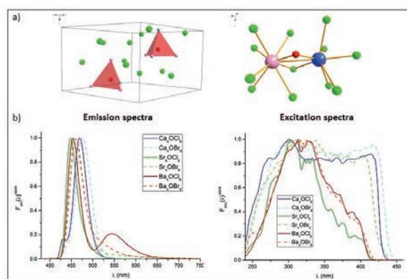
Fig. 1. a) Representation of the coordination of the two crystallographic sites M1 (pink) and M2 (blue) and the anion centered tetrahedra. b) Excitation and Emission spectra of the six  $M_4OX_6$  compounds at 5 K.
