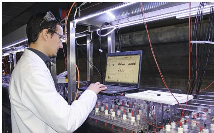
Research Assistant Maxime Blatter of the HES-SO uses electronic circuits to monitor the process and optimize electricity production and wastewater purification (Photo: Elsbeth Heinzelmänn).
