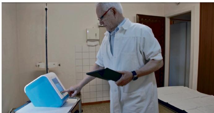
Abionic's abioSCOPE is a medical device that provides rapid diagnostic test results. It is composed of a fully automated fluorescent microscope and a mounting plate onto which is placed a single disposable IVD capsule. The abioSCOPE can be used by any healthcare professional and does not require extensive training. (Source: Abionic)
