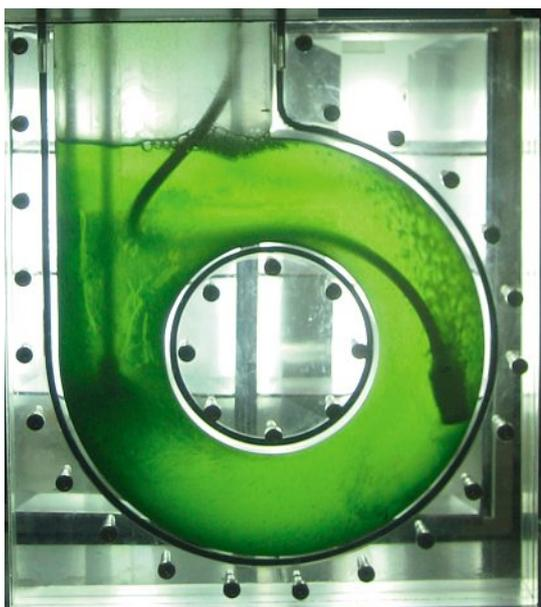
Fig. 3. Torus photobioreactor with micro algae cultivation.
