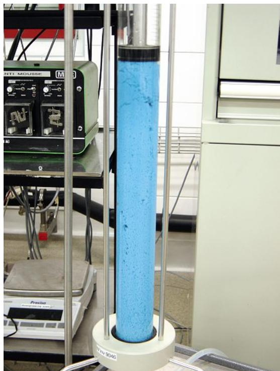
Fig. 4. Cu<sup>2+</sup> adsorption on a fixed bed of chitosan microbeads.
