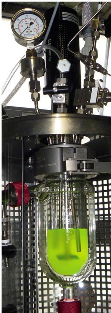
Fig. 1. Hydrogenation reactor.
