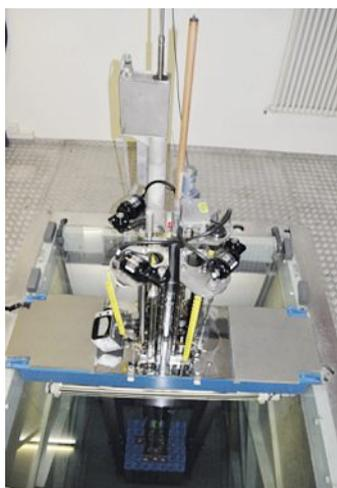
Nuclear reactor core at the University of Basel. The AGN-211-P is a light-water moderated swimming pool reactor with a power of 2 kW and a neutron flux of 3.8E+10 neutrons/cm<sup>2</sup>/s (photo by G. Testa).
