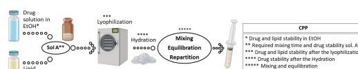
Figure 1. Process flow chart and the critical process parameters that could affect the quality of the final product using (A) a standardized method and (B) the dual syringe method.
