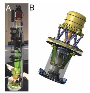
Laboratory setup to test the laser and optical components of the LIMS (A) and instrument flight design as shown by the CAD drawing (B). For illustrative purposes the TOF mass analyzer has been placed directly under the optical cage. Under operating conditions, it is mounted in a vacuum compartment. The sample introduction system will be attached to the bottom of the flight design.
