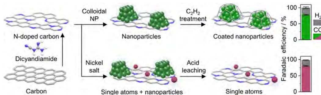
Figure 1 Synthesis of distinct nickel species on nitrogen-doped carbons and corresponding Faradaic efficiencies in the electrochemical CO 2 reduction reaction.
