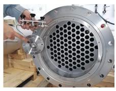
Size comparison between a test device for measuring the permeability of hydrogen selective membranes and a small industrial reactor. In industrial membrane reactors, the membranes are designed as tube bundles, while a flat design (a flat membrane is inserted at the location indicated by index finger) is chosen for scientific characterisation. The need for cheap membrane materials is obvious.
