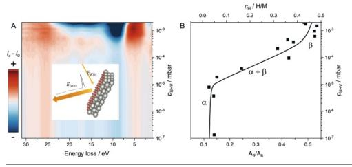
Left: Principle of reflecting electron energy loss spectroscopy (REELS) inset. Left and right: REELS difference spectra of the downstream surface of a vanadium membrane at 100 °C exposed to incrementally increased hydrogen pressure as 2D-contour plot showing the continuous change of the spectra upon hydrogen uptake particularly strong at 5 and 8 eV. The corresponding pressure surface composition isotherms are derived from the area ratio at these loss energies and the measured permeate pressure.
