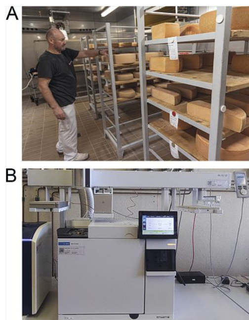
Agroscope's experimental cheese factory (A), Agilent 8890 gas chromatograph coupled with a flame ionization detector and a PAL3 autosampler in headspace mode (B).
