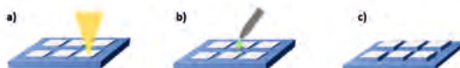
Figure 1. a) Exposure of specific regions to the electron beam (gray areas) promotes surface passivation and as result, a nanomasks array is fabricated. The blue area represents the area that was not exposed to the electron beam. b) Nanomasked samples subjected to chemical etching. c) Upon chemical etching, only the non-masked sample regions are eroded whereas the masked areas remain intact.
