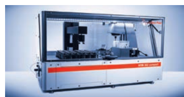
HTR Compact: rheometer autosampler for high sample throughput.
