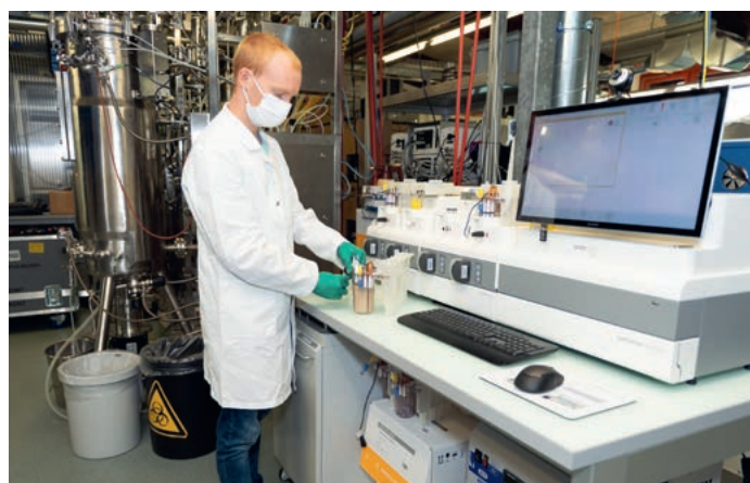
Fig. 1. ambr 250 modular used for the first scale-up step of the upstream processing of SARS-CoV-2 VLP production in the technology room of ZHAW's Center for Biochemical Engineering and Cell Cultivation Techniques (Photo: Patrick Cipriani)
