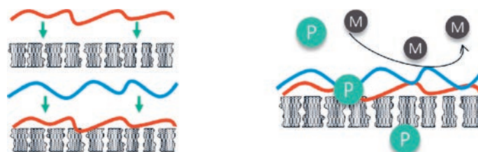
Fig. 1. Deposition of a polycation (red) and polyanion (blue) on a porous ultrafiltration membrane (left) and a schematic description of the transport mechanisms of a LbL membrane during phosphorous recovery from acidic disintegrated sewage sludge (right, P = phosphorous, M = metal ion).
