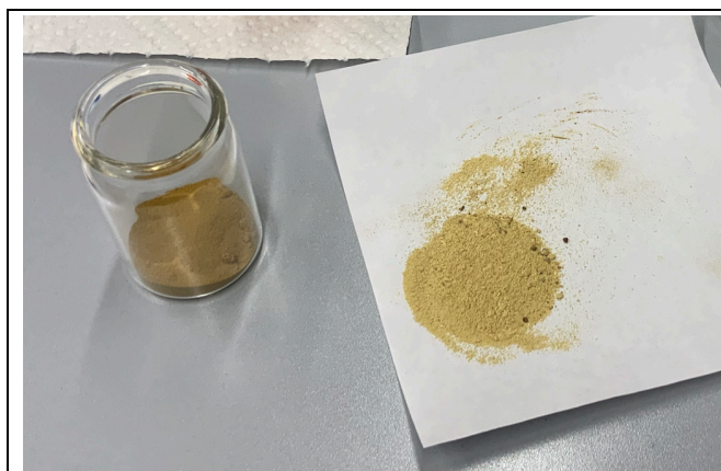
left: sample recrystallized from EtOH; right: partially undissolved material left on filter
