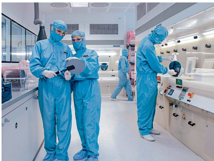
Fig. 1. Chip manufacturing requires high purity chemicals. Production and analytics is performed in a 'clean room'. The above picture shows a BASF test lab for cleaning chemicals used for silicon wafers.
