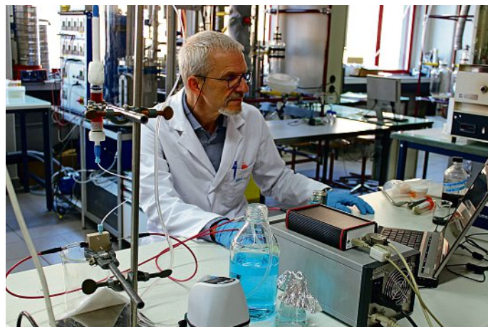
Experimental set-up for the measurement of breakthrough curves. Prof. Simon Crelier is configuring the fiber optics spectrophotometer used for concentration measurements in the effluent. The detection cell can be seen after the adsorbent fixed bed in the bottom left of the picture. (Photo Elsbeth Heinzelmänn)
