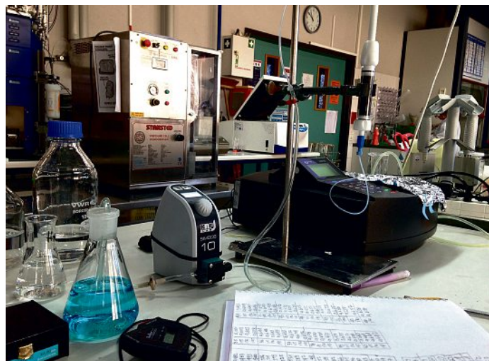
A flask of contaminated effluent, a pump, a column with a fixed bed of adsorbent and a detector: a simple laboratory set-up can provide very useful information on adsorbent capacity and mass transfer. (Simon Crelier HES-SO Sion)
