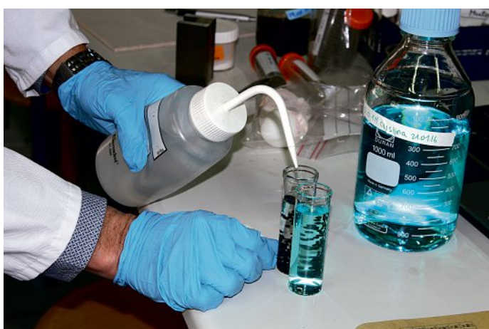
Suspending composite chitosan/maghemite magnetic adsorbent particles in a copper sulphate solution. (Photo Elsbeth Heinzelmann)
