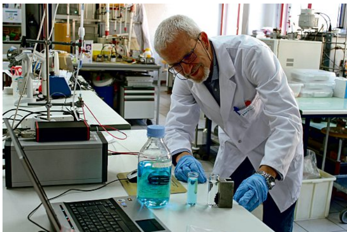
Separating magnetic adsorbent beads from treated effluent containing copper ions. The original blue-colored copper sulphate solution can be seen in the left-hand tube. After complete removal of the metal ions, the beads can be sequestered using a simple magnet, the decontaminated liquid released, the copper released in a more concentrated form allowing proper reuse and the adsorbent regenerated. (Photos Elsbeth Heinzelmann)
