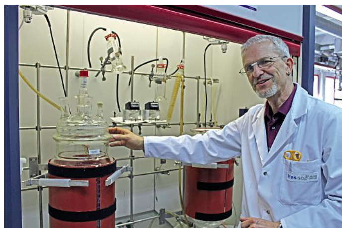
UAS professor Simon Crelier, who teaches downstream processing and enzyme technology, presents the 20-litre stirred glass reactors with temperature control for anaerobic digestion at the Biotechnology Unit of the Life Technologies Department. Photo: Elsbeth Heinzlmann.
