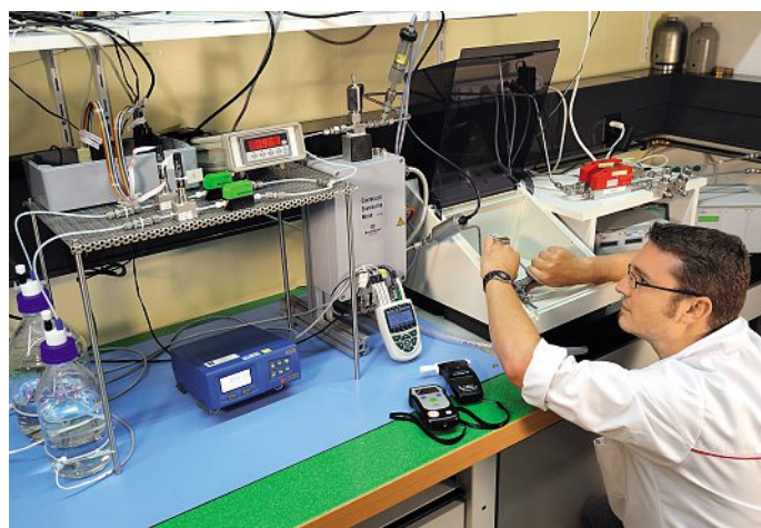
The generator for wet breath-alcohol analysis built at METAS.
