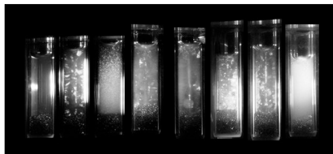
Illustration 1: A set of samples characterized by increasing volume fractions (from left to right: 3.8%, 5.7%, 11%, 15%, 21%, 27%, 30% and 34%). Presence of a crystalline phase is evidenced by the iridescence.
