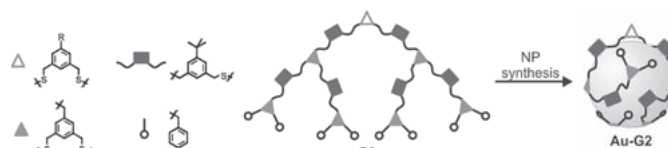
Figure 1. Second generation dendrimer (G2) and G2-stabilized Au NP; R = t -butyl or acetylene-TIPS.
