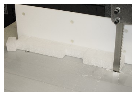
Ice core sample cutting with a band saw (photo: A. Ciric).
