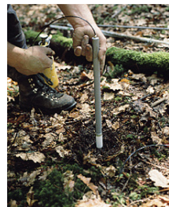
Installation of a lysimeter
