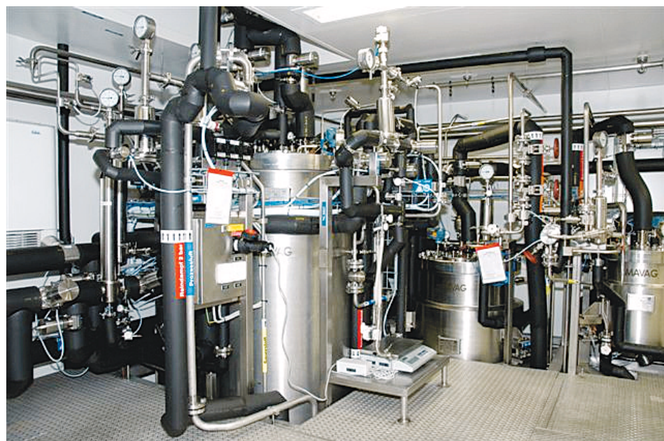
Fig. 3. 1000 l High-performance bioreactor for the production of biopharmaceuticals
