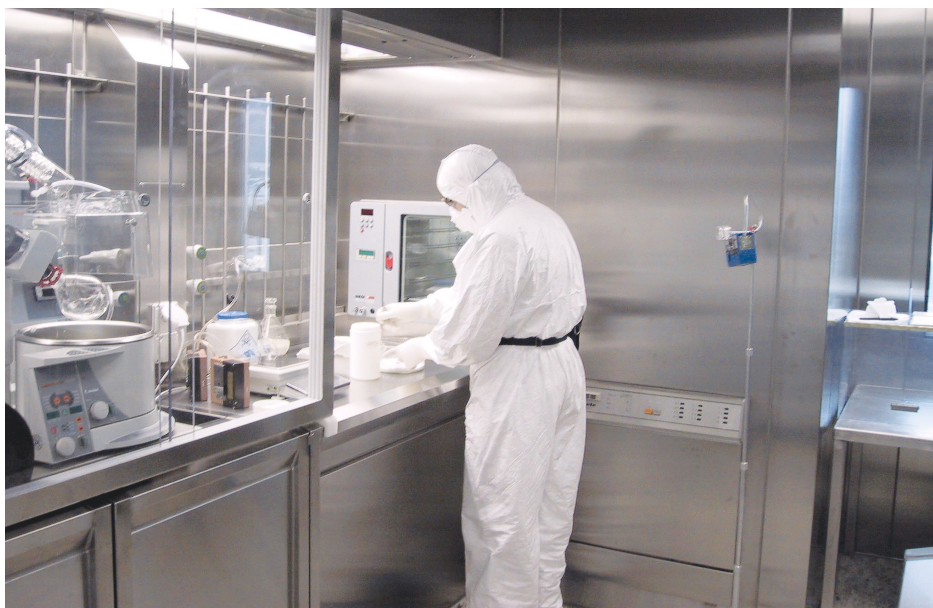
Fig. 5. A fully equipped qualified clean room with air-lock system is available on top of building E-38 for kg-quantities under GMP or also suitable for handling of highly active compounds
