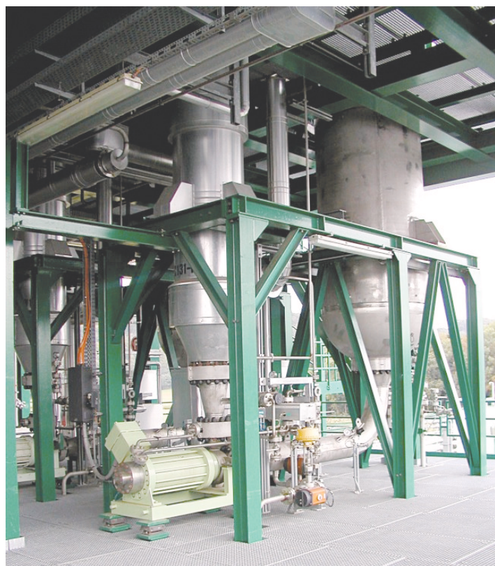
Fig. 2. Loop reactor with circulation pump and heat exchanger
