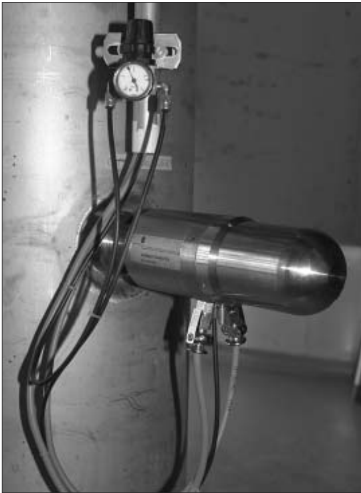
Fig. 3. Measuring instrument 'Labasys® Control Ex' for inline monitoring of particulate product flows.
