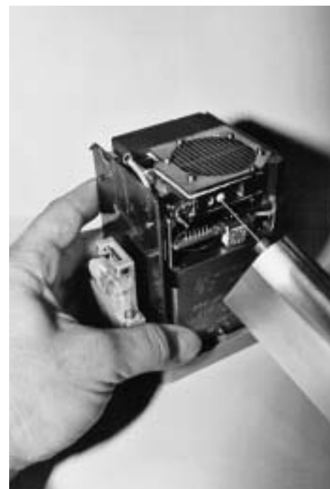
Fig. 2. Miniaturized bioreactor with two syringes for the sampling and the sample bottles. The cultivation chamber is on the top. The inspection window is located on the right upper side. The bottom structure contains the fresh and the used medium. Total height 8 cm.
