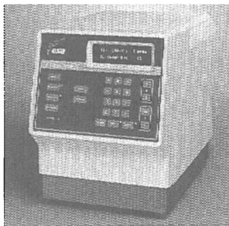
Fig. 10. ESA Coulochem II Multielectrode Detector for HPLC featuring DC, Pulse, and Scan modes of operation
