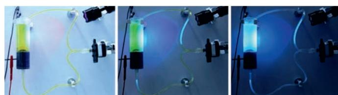
Fig. 4. Left: Start of discharging process of Lamy T 10 Neon Lime in acidified 1 M ZnSO<sub>4</sub> under daylight; middle: during discharging under UV light; right: completely discharged hybrid flow battery under UV light.
