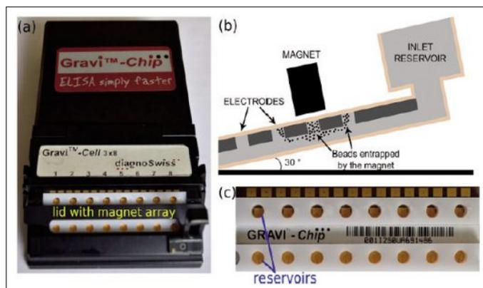
a) GRAVI<sup>TM</sup>-Cell device with an 8-microchannel chip tilted at 30°. b) Cross-section along the microchip showing magnetic beads trapping. c) GRAVI<sup>TM</sup>-Chip comprising 8 microchannels, inlet reservoirs at the top and outlet ones at the bottom.
