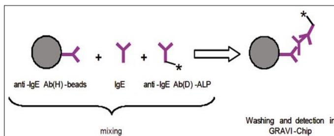
One-step sandwich ELISA: immunocomplex is formed by secondary anti-human-IgE antibodies Ab(H) immobilized on magnetic beads surface, IgE antibodies present in the sample, and by secondary anti-human-IgE antibodies Ab(D) labeled with enzyme alkaline phosphatase (ALP). The electrochemically active substrate of ALP is used for detection.
