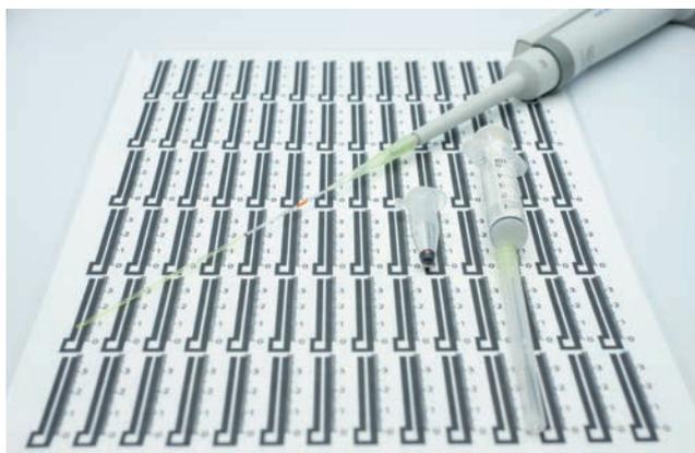
Apply a drop of serum through a special capillary into a paper channel and get the result!
