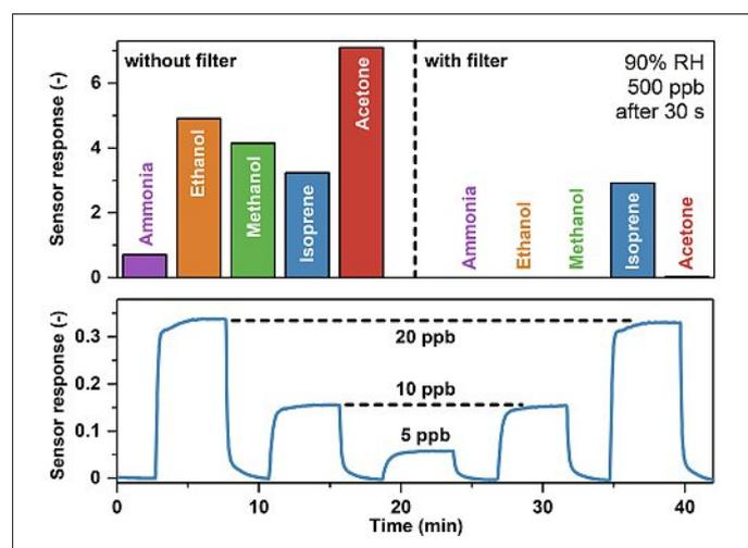
Response of the Pt-doped  $\text{SnO}_2$  sensor without (top left) and with activated alumina filter (top right) to 500 ppb of breath-relevant analytes at 90% RH. Response of the filter-sensor system to ultra-low isoprene concentrations of 5, 10 and 20 ppb at 90% RH (bottom). Adapted with permission from van den Broek *et al.*, *ACS Sens.* **2018**, *3*, 677. Copyright (2018) American Chemical Society.
