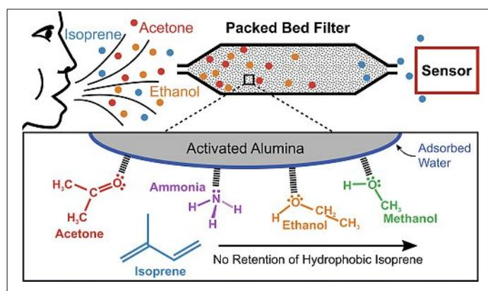
Isoprene detector based on an alumina-powder filter to retain hydrophilic compounds and a highly sensitive Pt-doped  $\text{SnO}_2$  sensor to quantify isoprene concentrations. Adapted with permission from van den Broek *et al.*, *ACS Sens.* **2018**, *3*, 677. Copyright (2018) American Chemical Society.
