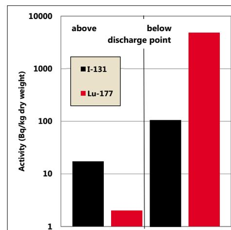
Load of sewer sludge in the vicinity of a hospital centre (notice the logarithmic y-axis).
