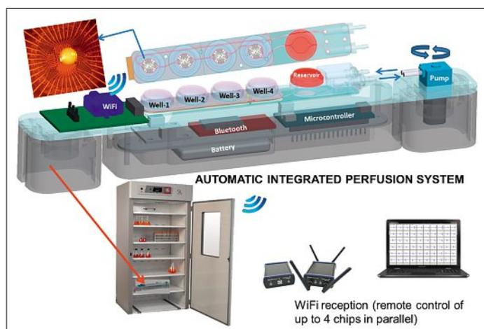
Scheme of the stand-alone BioChip showing the different parts of the integrated system. A miniature peristaltic pump allows the perfusion of the culture medium from the reservoir to the different wells through a Bluetooth remote control. The insert shows a 3D neural culture derived from hESCs placed onto the multi-electrode array. Recordings of electrical signals are sent to the acquisition software through a WiFi transmission. Image: Luc Stoppini.
