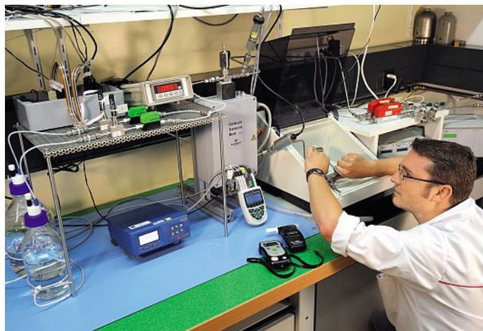
The generator for wet breath-alcohol analysis built at METAS.
